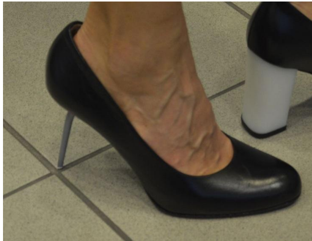
Fig. 9: Test shoe with the newly developed heel attachment variant
