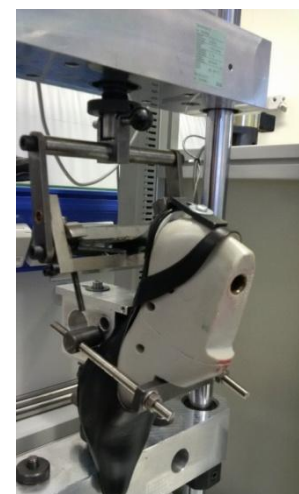
Fig. 8: Procedure for dynamic testing of heel attachment
