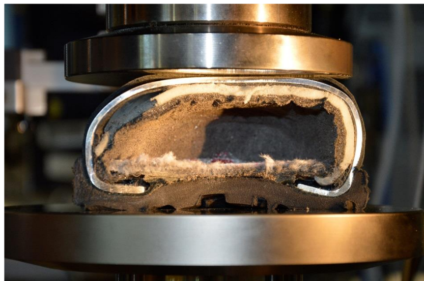
Fig. 6: Compression test according to ISO 20344 – here 5 kN
