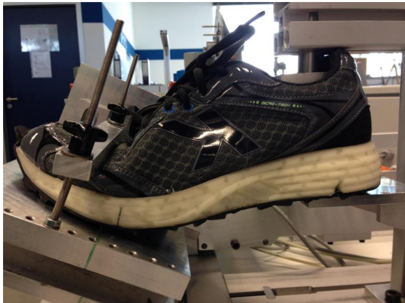
Fig. 1: Sole of a 3D-printed sports shoe produced in the ADDFactor EU Research Project in 2014 undergoing endurance testing on a PFI flexibility testing machine
