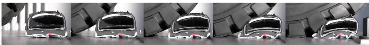
Fig. 5: Descent of toe caps into the sole with increasing force on being run over (Concluding report of AiF Project 17636)
