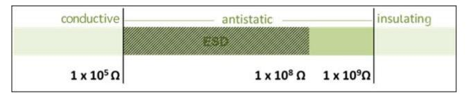
Antistatic DIN EN ISO 20345 – Personal Protection - Requirement 1 x  $10^5$  < x < 1x  $10^9$  Conductive DIN EN IEC 61340-4-3 Equipment Protection or DIN EN IEC 61340-5-1 Workplace Measurement - Requirement 1 x  $10^5$  < x < 1 x  $10^8$
