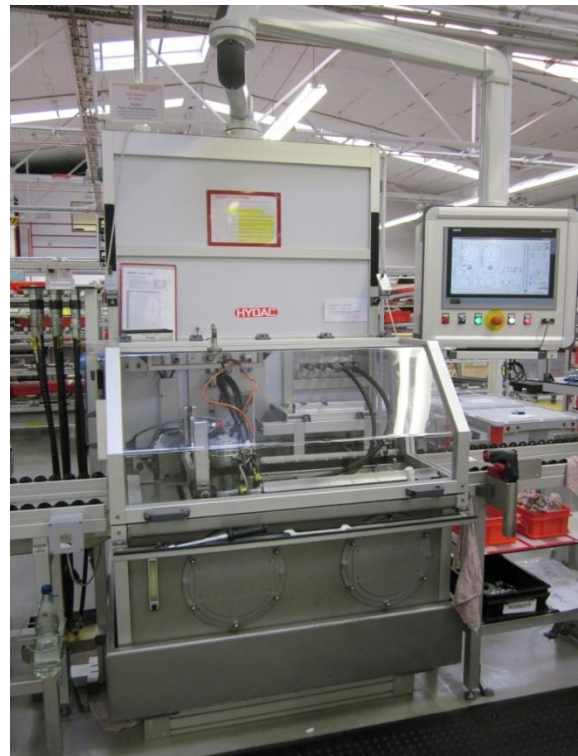
Closed assembly test bed for motors, pumps, and valves developed jointly by PFI and the Technology and Process Development department of HYDAC
