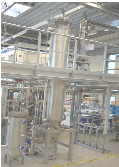
PFI engineering lab scale plant for methanation and power-to-gas pilot plant built at Pirmasens Energy Park
