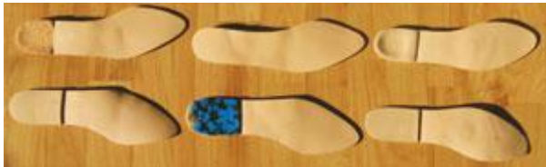
Fig. 8a and b: Test footbeds for “fashion” shoes
